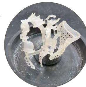
Ranger has also learned a few tricks to further reduce his costs. For instance, he designs the support sprue bar larger than necessary, uses it as a sprue, then piggybacks cases and casts and invests multiple cases simultaneously, saving labor and material.
